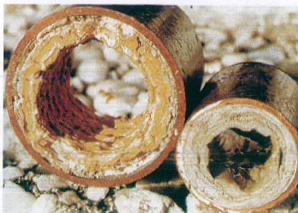
Exhibit 8.4: Scale formation in boilers
