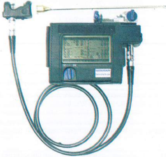
Exhibit 6.16: A typical portable electronic combustion analyzer
