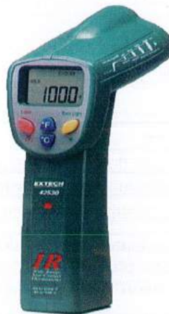
Exhibit 6.2: Typical infrared thermometer for non-contact temperature measurement
