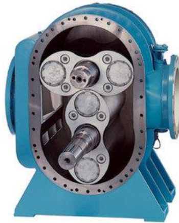
Exhibit 10-5: Function mechanism of positive displacement blower
