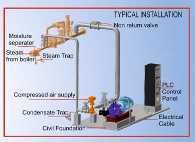
The Pressure Reducing Turbine (PRT®) is a special purpose steam turbine to bypass the Pressure Reducing Station (PRS) while simultaneously generating power.
