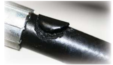
Real life problem 3 Damaged Pneumatic Tools
